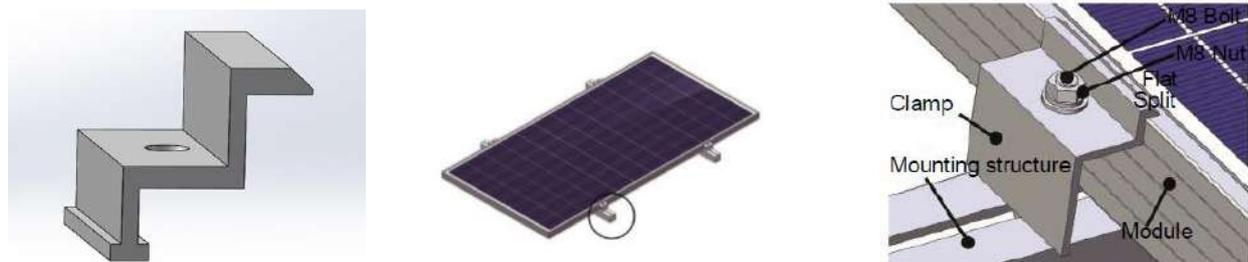
**\*\* The required length for each clamp is minimum 50 mm, and wall thickness of its upper part is no less than 5mm**
