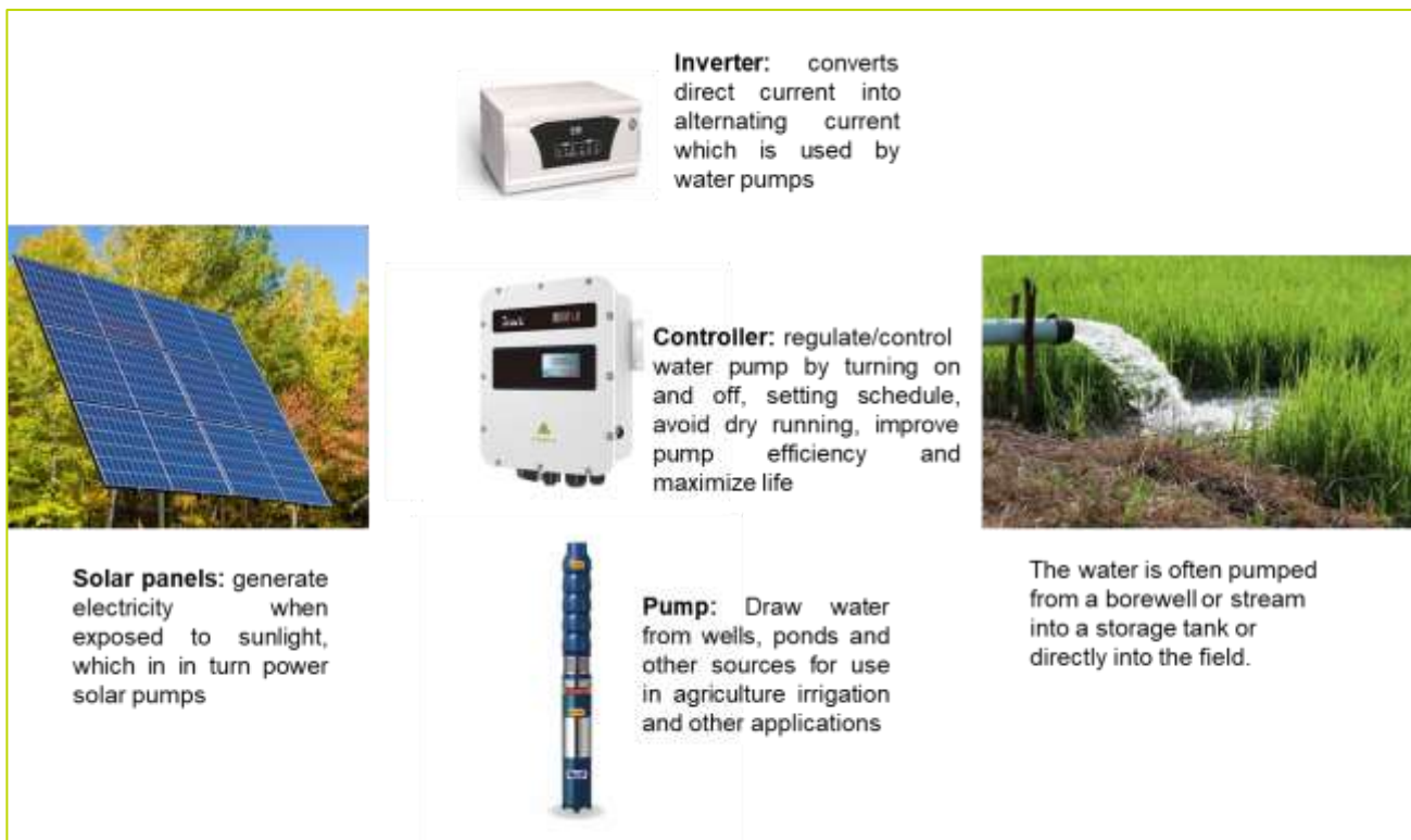
Figure 61: Key components of solar water pump system
